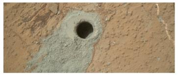
Figure 12. Curiosity's tools include a drill to obtain subsurface samples. Credit: NASA/JPL-Caltech/MSSS.
